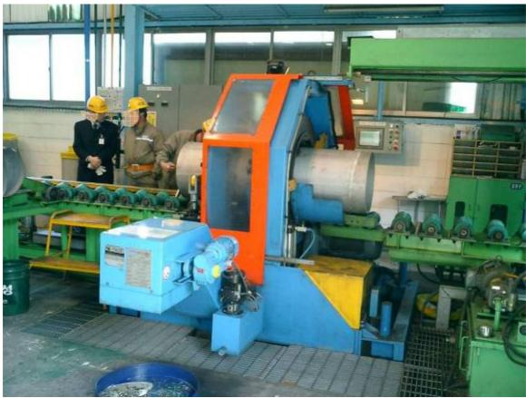
The CTA model is designed for production or prefab workshops. It allows cutting and beveling tube sections at the right length. The cutting is square and the bevel angles are very precise. The cold machining process gives a clean surface finish and does not affect the pipe material features.
