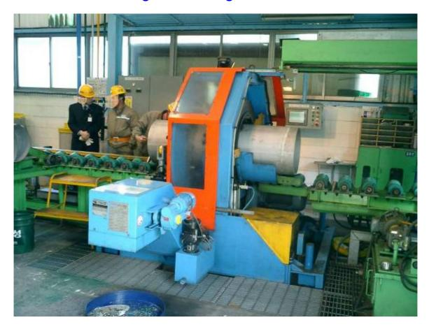
The CTA model is designed for production or prefab workshops. It allows cutting and beveling tube sections at the right length. The cutting is square and the bevel angles are very precise. The cold machining process gives a clean surface finish and does not affect the pipe material features.
