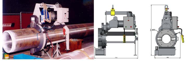
The TNO beveling machines are especially designed to fit your piping or tubing prefab application on site or in workshops. These machines sever and bevel heavy wall pipes faster than any other machine. They allow to save man hours by avoiding grinding operations, flame cutting, difficult handling and setting of pipes on a lathe. They are transportable, rigid, fast and accurate.
